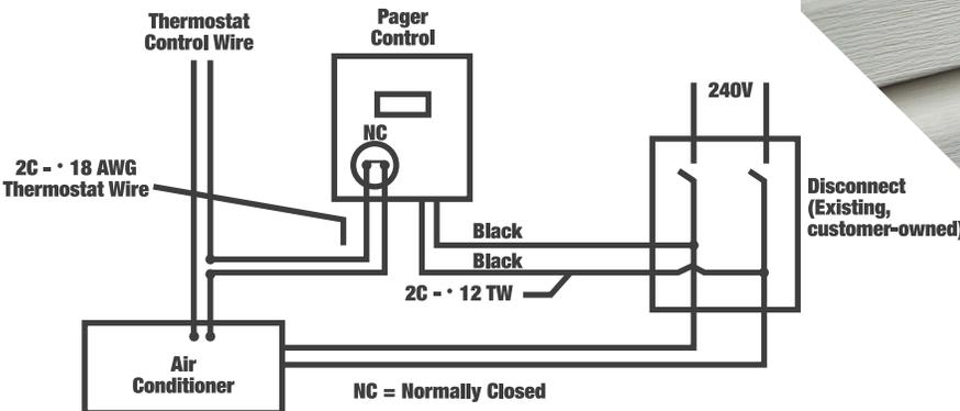
Electrical specifications for the LCR include voltage: 240 VAC (+10% -20%) and frequency: 60 Hz ( $\pm$  2%).
