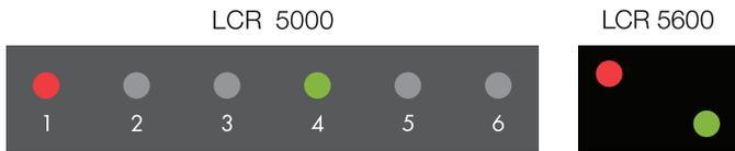
When the LCR 5000 is controlling the compressor, LEDs 1, 4 and 5 will be lit on older models. On newer models, only LEDs 1 and 4 will be lit. At all times, disregard LED 5; its status is not relevant to the operation of the LCR. When the LCR 5600 is controlling the compressor, a red LED on the left side and a green LED below and to the right will be lit.
